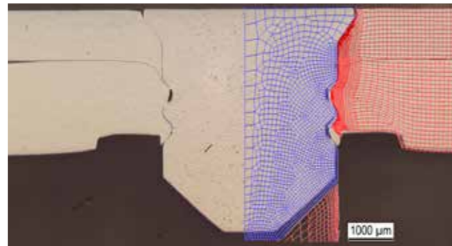
Al-VSN connection with a total sheet thickness of 3.1 mm (sheets: EN AW-6111 PX, self-piercing rivet: AA 7068 T651)
