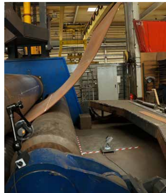
Measurement of sheet metal forming with the help of developed process monitoring.
