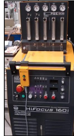
Cutting appliance Hi Focus 160i with gas mixer
