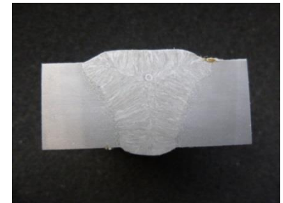
Macrosection EG weld seam, t = 18 mm
