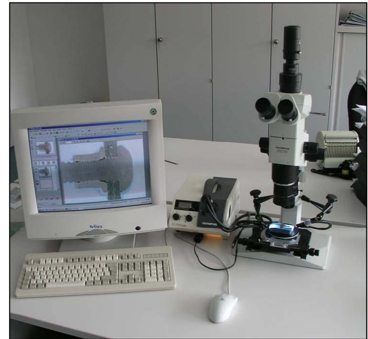
Photograph and detailed examination with stereo-microscope Olympus SZX12 of macro-polished sections
