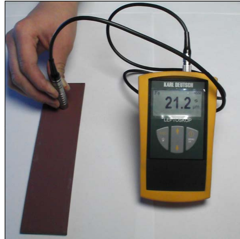
Coat thickness measuring with the Leptoskop 2042 with Fe-sensor ( 0-3.000 \mu\text{m} )
