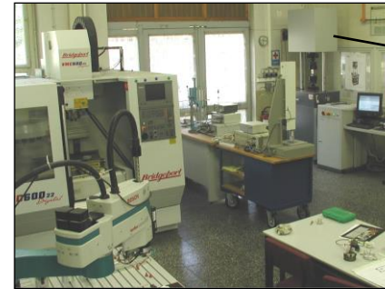
High frequency pulsator in production engineering lab during high cycle fatigue tests
