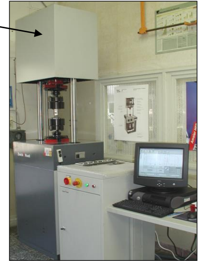
High frequency pulsator in production engineering lab during high cycle fatigue tests
